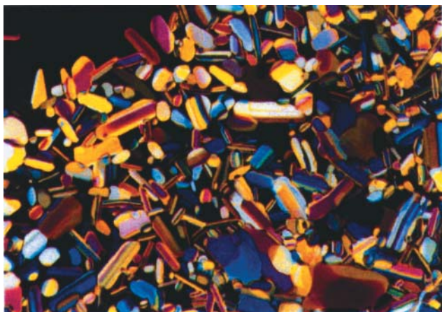
Fig. 2 Optical texture of the crystal B phase exhibited by compound 7a under crossed polarizers at 189.4 °C (on heating).
